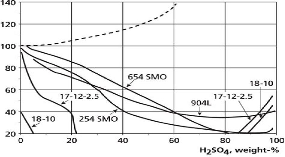
Isocorrosion diagram, 0.1 mm/year, for austenitic stainless steels in naturally aerated sulphuric acid of chemical purity. Broken-line curve represents the boiling point.
