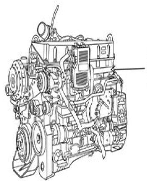
The engine dataplate is located on the rocker housing which is located on the fuel pump side of the engine.
