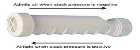
When negative pressure occurs, the Hep<sub>v</sub>O<sup>®</sup> valve partially opens and closes until sufficient air flow is drawn to maintain it open. Once equilibrium is reached, the valve closes. Positive pressure in the downstream system applies pressure to the valve keeping it closed.
