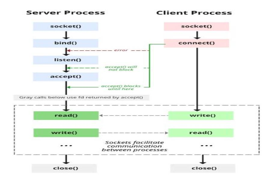
State diagram for server and client model of Socket
