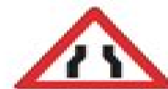
W328 Barabara nyembamba pande zote
