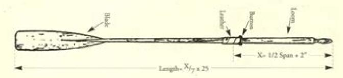
I nboard length of the loom equals 1/2 the span between the oarlocks + 2".
