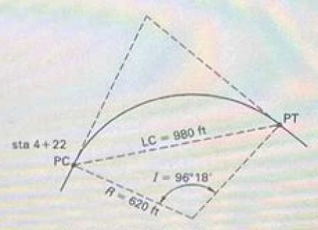
The curve radius, R, is 620 ft. With stationing around the curve, the stationing of the point of tangent, PT, is most near to
