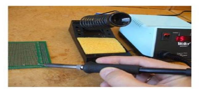
Soldering is process of joining two metals together with soldering iron by the use of a solder to form a dependable electrical joint.
