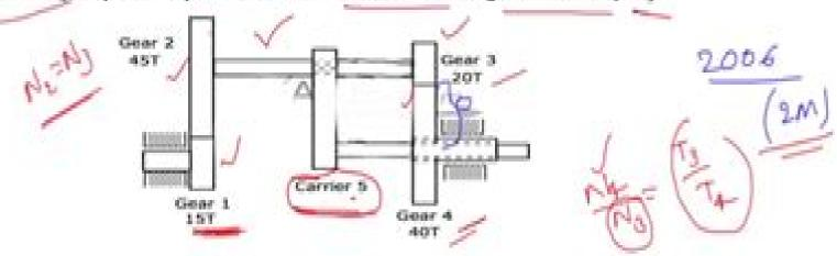
74. What is the relation between the angular velocities of Gear 1 and Gear 4?
