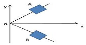
Strain gauges do not respond to shear strains. However the relationship between shear and normal strains can be utilized to obtain from a strain rosette an output directly proportional to the shear strain in the surface.
