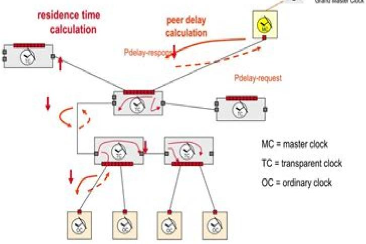
Two calculations: residence time and peer delay All nodes measure delay to peer TC correct for residence time (HW support)
