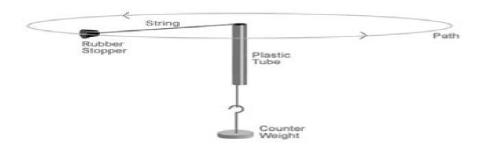
Let M be the mass of the counter weight and m the mass of the rubber stopper. Newton's 2nd law for the stopper is
