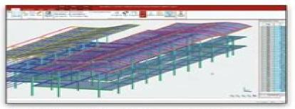
Physical modeling capabilities enable engineers to better participate in 83M workflows, automatically generating the analysis models for both simple and complex structural analysis.
