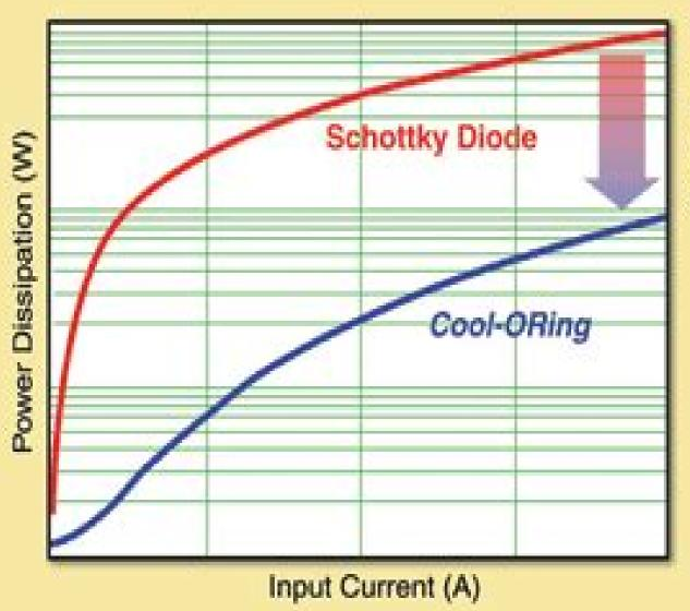
10X Reduction in Power Dissipation Reducing Thermal Management Overhead
